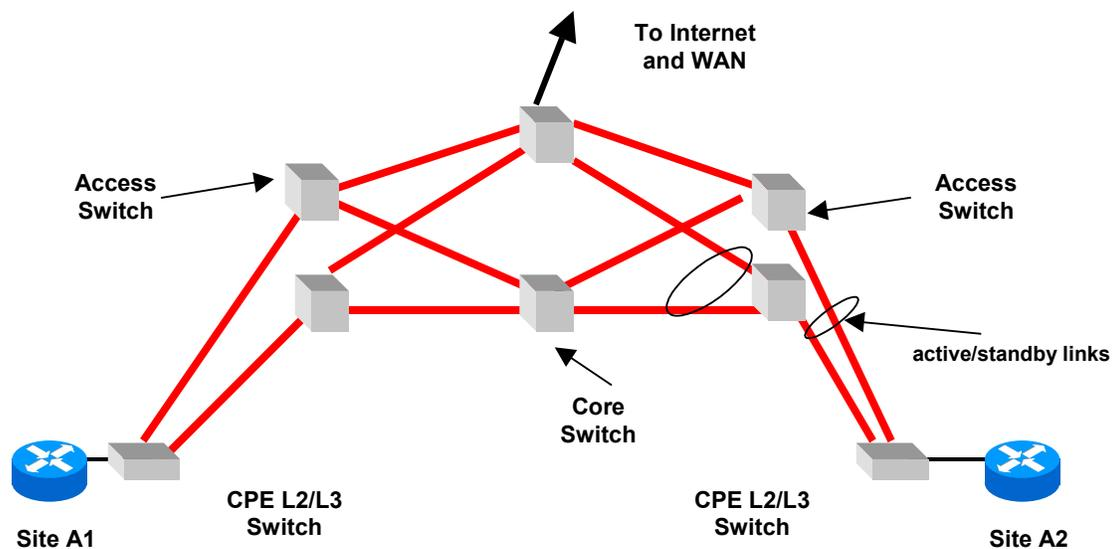
**Figure 3: MAN based on IP over Long Haul Ethernet**
