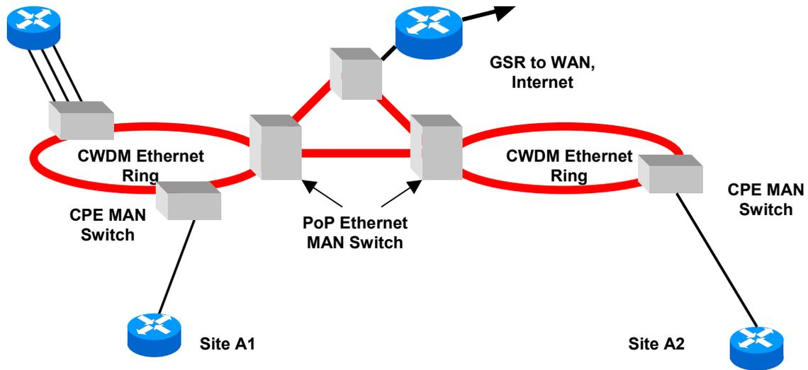
**Figure 4: MAN based on IP over Long Haul Ethernet and CWDM Rings**
