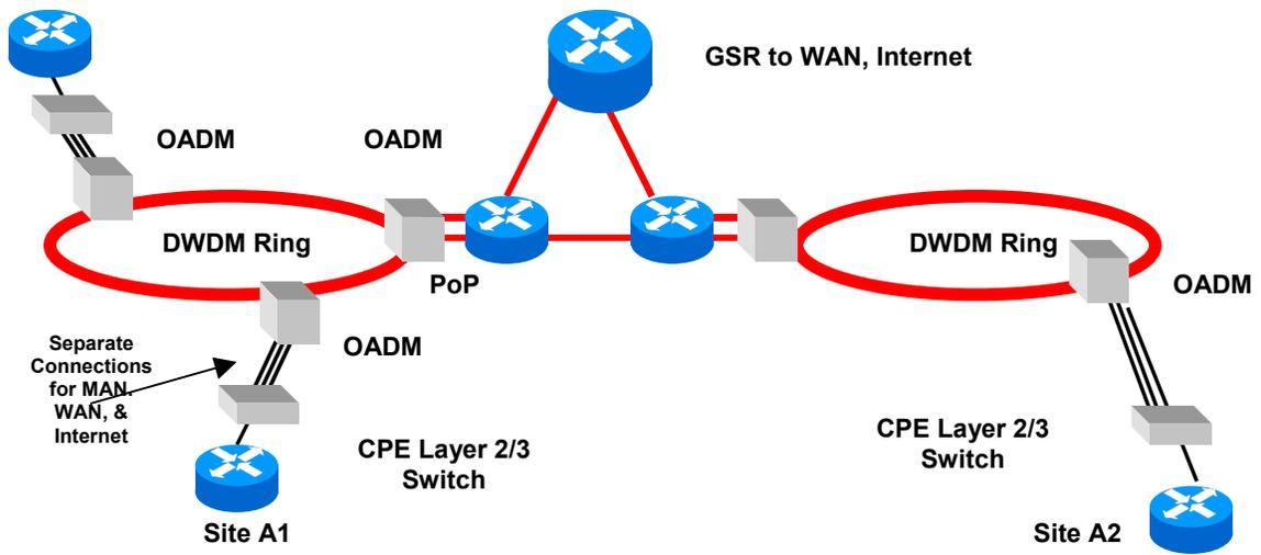
**Figure 5: MAN based on IP over DWDM Rings**
