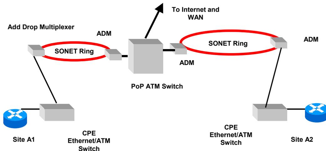
**Figure 2: MAN based on ATM/SONET/SDH TLS**
