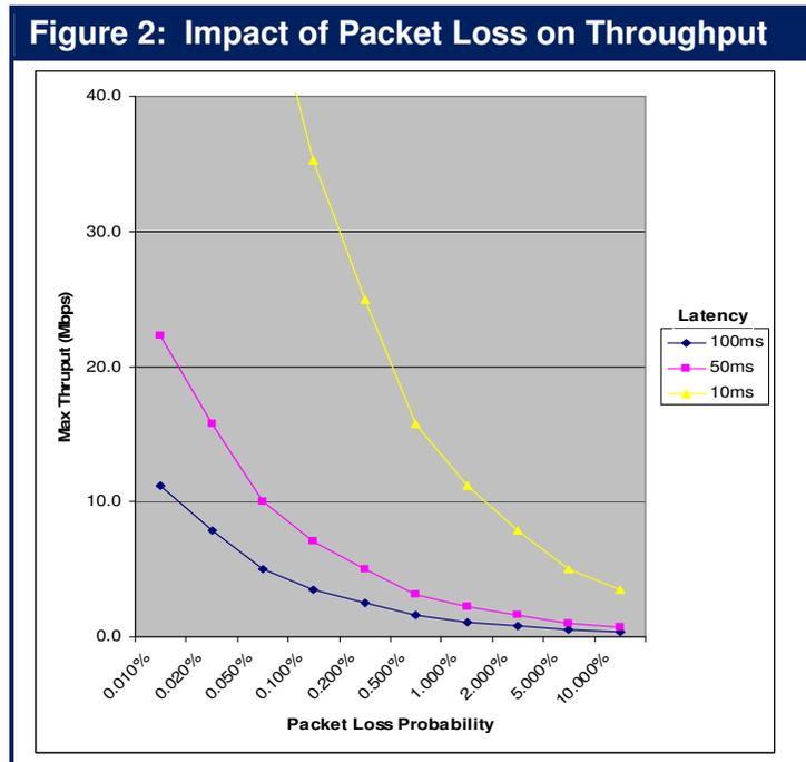
For example, on a WAN link with a 1% packet loss and a round trip time of 50 ms or greater, the maximum throughput is roughly 3 megabits per second no matter how large the WAN link is.
